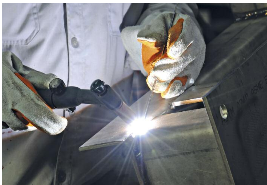
Manuelles Wolfram-Inertgas- (WIG-)Schweißen © iStock.com/Lekyum
